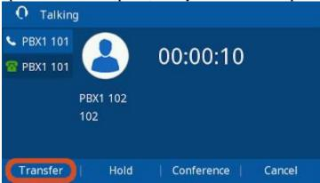
• To Complete The Transfer: Press the (Transfer) Button or the Transfer Softkey.
