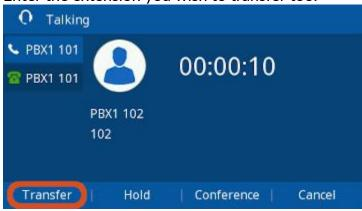
• Press the (Transfer) Button or the **Transfer** Softkey again to complete the Transfer.
