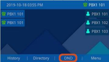
• When DND is enabled you will see a DND icon on top of the screen, and a "DND Mode!" Message at the bottom. The Bottom Message may cycle through other messages like "Headset Mode" etc.
