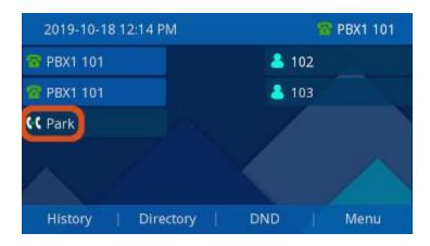
• The Caller will be placed in a parking slot, and the slot number will be read back to you, press the (Transfer Button) or Softkey again to complete the transfer to parking.
