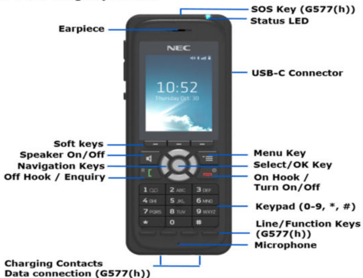
Figure 4: Elements of the G277/577 (Front View)
