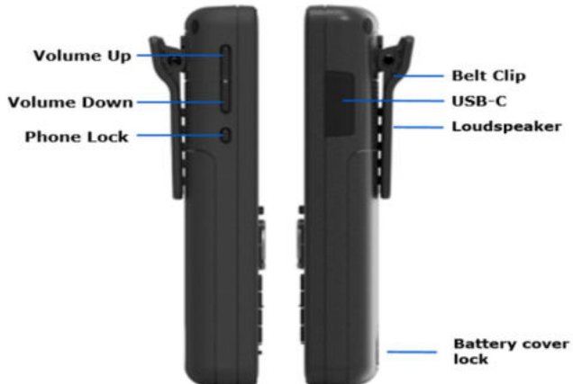
Figure 5: Elements of the G277/577 (Side Views)
